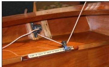
an Enterprise and mounted them horizontally on the top surface of the tank, this provided an easy solution as it obviated the need to find a separate cleat.
