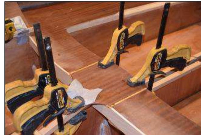
The centre piece of the thwart is clamped in place
