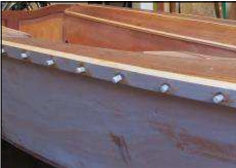
Rubbing beads are glued and screwed. When set the screws are removed and the holes plugged making a nice row of cannon ports!!! (until faired off)
