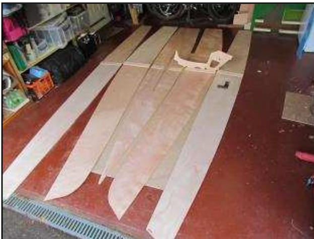
The next stage is making up batters from the scrap ply followed by lots of glueing to form the major parts of the hull
