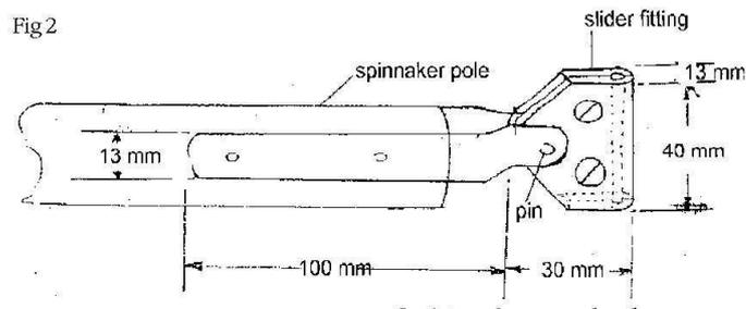
The slider can be made from pieces of nylon and the slide fastenings to the pole out of stainless steel. A pin with circlip joins the 2 parts together allowing the slider to pivot freely when the pole is stored.
