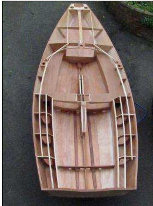
The thwart is constructed to the reverse curve design
