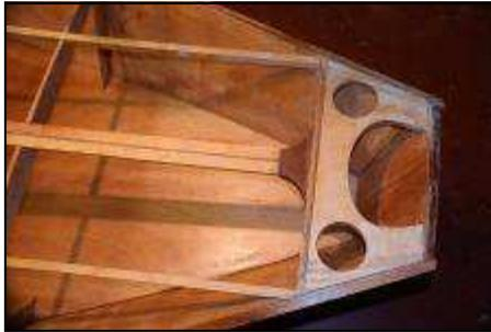
I have now added some hardwood to the rear of the spinnaker chute to provide a solid base for the jib plate, with the whole assembly being designed to take the loading on the rigging
