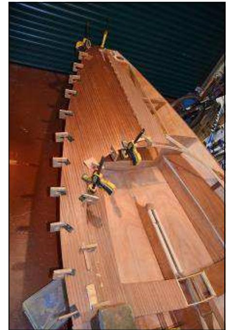
The decks are fitted using simple plywood clamps and wedges (nice and cheap) plus a few of the real things!
