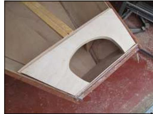
The components of the central chute can now be added, but oops Part 44Z is not exactly correct and I think I will have to add a bit of hardwood behind the mouth to provide a solid surface to screw the jib plate onto
