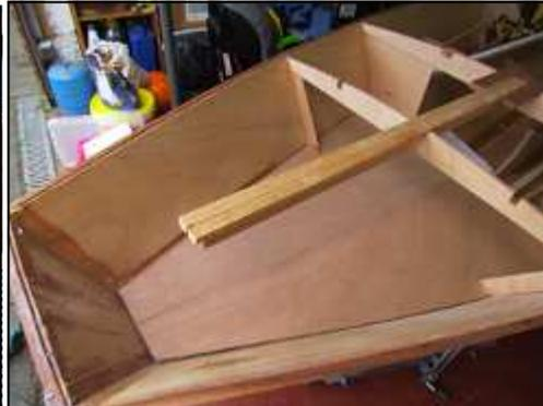
The lower fore deck is installed in two halves resting on a central bearer (not in the plans). It comes slightly oversize and needs to be planed down
