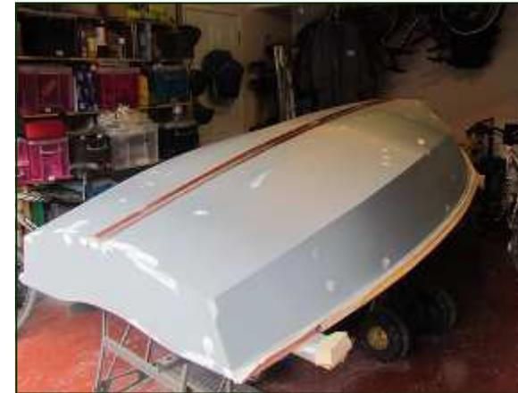
The keel is on and the filling and fairing are nearly complete (now I know why people send their boats to the paint shop!!). When done the top coat is applied, then its a quick turn over to varnish the decks and interior. All is now ready to start screwing the fittings on
