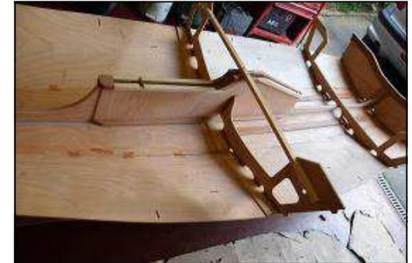
Some floor battens are inserted and glued as they are easier to reach now
