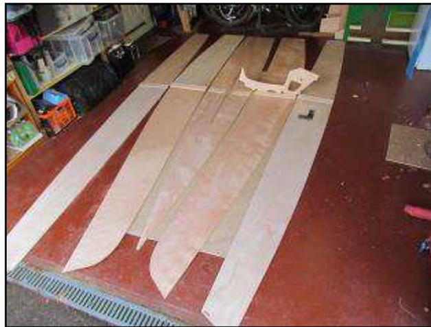
The next stage is making up battens from the scrap ply followed by lots of glueing to form the major parts of the hull
