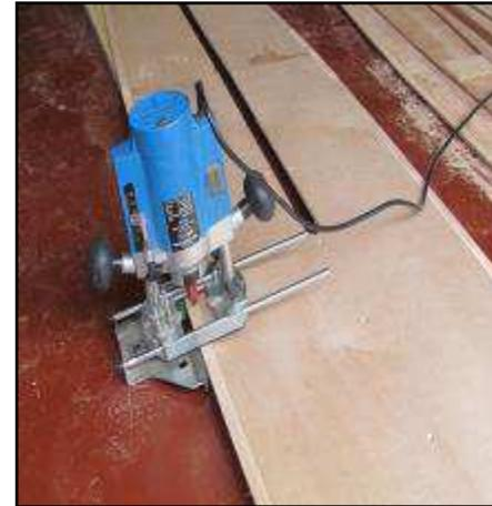
Then to save time and effort on fairing the hull at a later stage the edges are routed out to a shallow depth just sufficient to accept the tape
