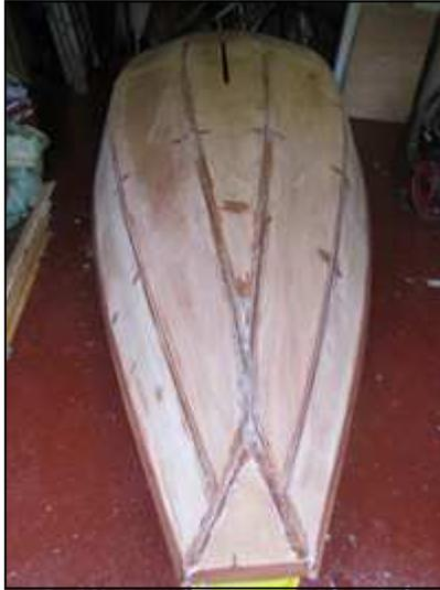
The hull is now taped and secure
