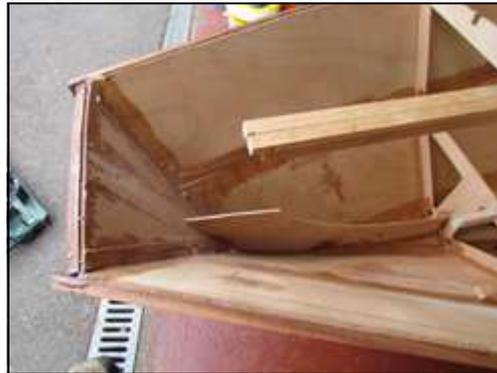
Now we can cut away the stem prior to constructing the central spinnaker chute
