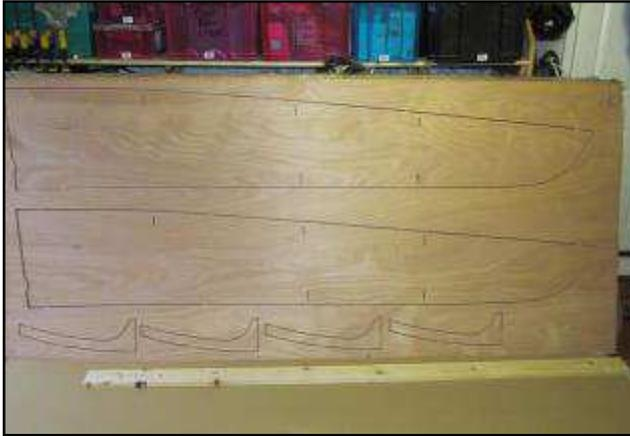
The ply sheets arrive, pre-cut by router and are quickly and easily removed. I was amazed that within a couple of hours I had most of the parts ready to assemble. When I built 3838 it took me days to scale up the drawings onto ply sheets and cut out with a jig saw
